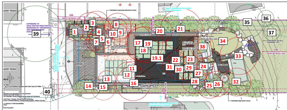
Figure 1: showing proposed design footprint & tree removal plan
