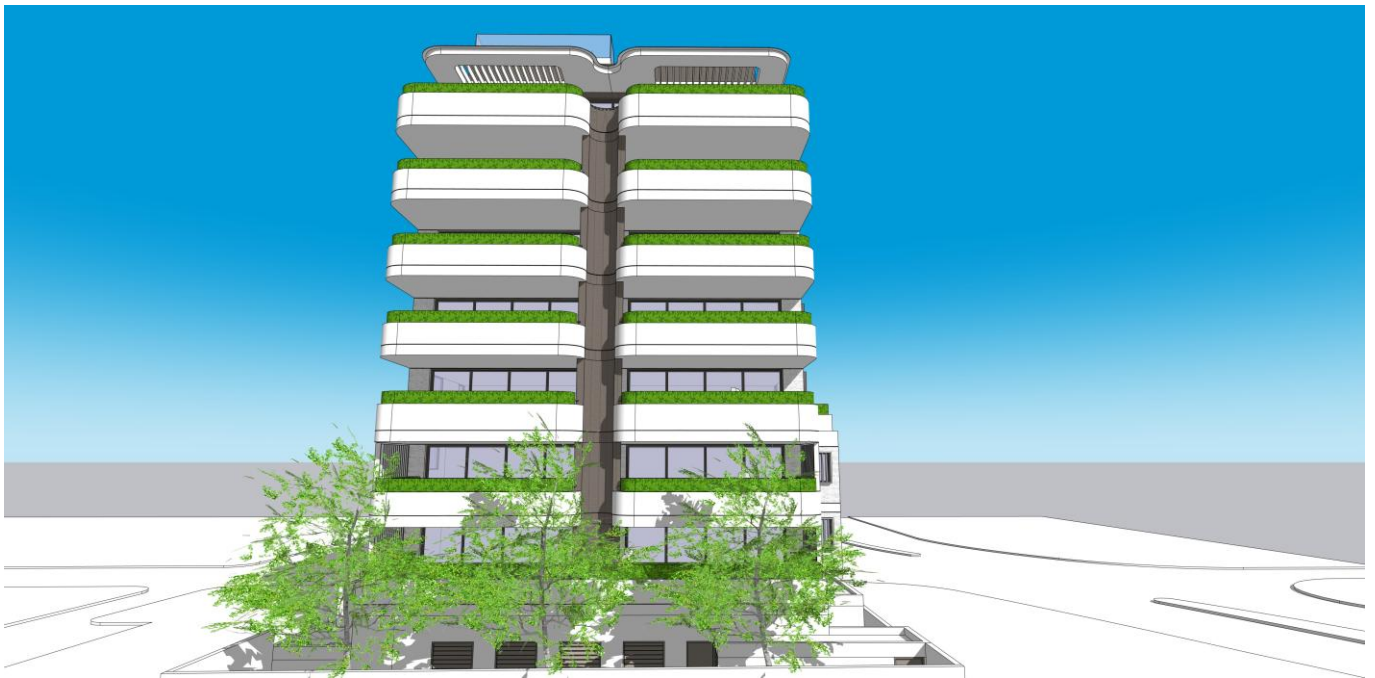
Above: The north façade is divided into 2 vertical forms with a recess between the balconies. Planters provide privacy to neighbouring buildings
