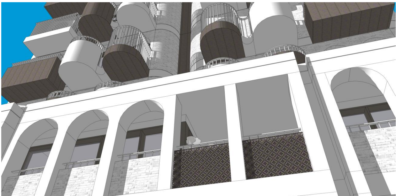
Above: Raglan St façade detail in copper and face brick
