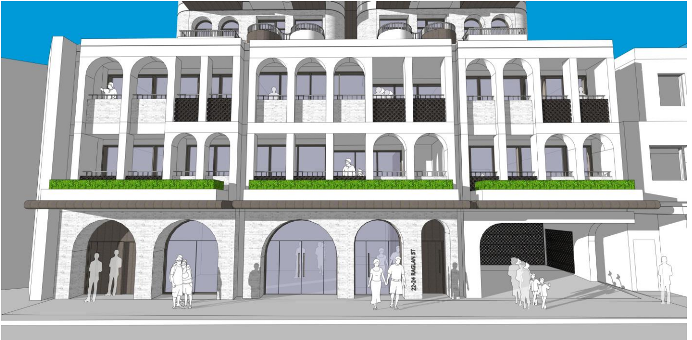
Above: 3-storey podium in off-white face brick with arched and rectangular openings in deep masonry walls
