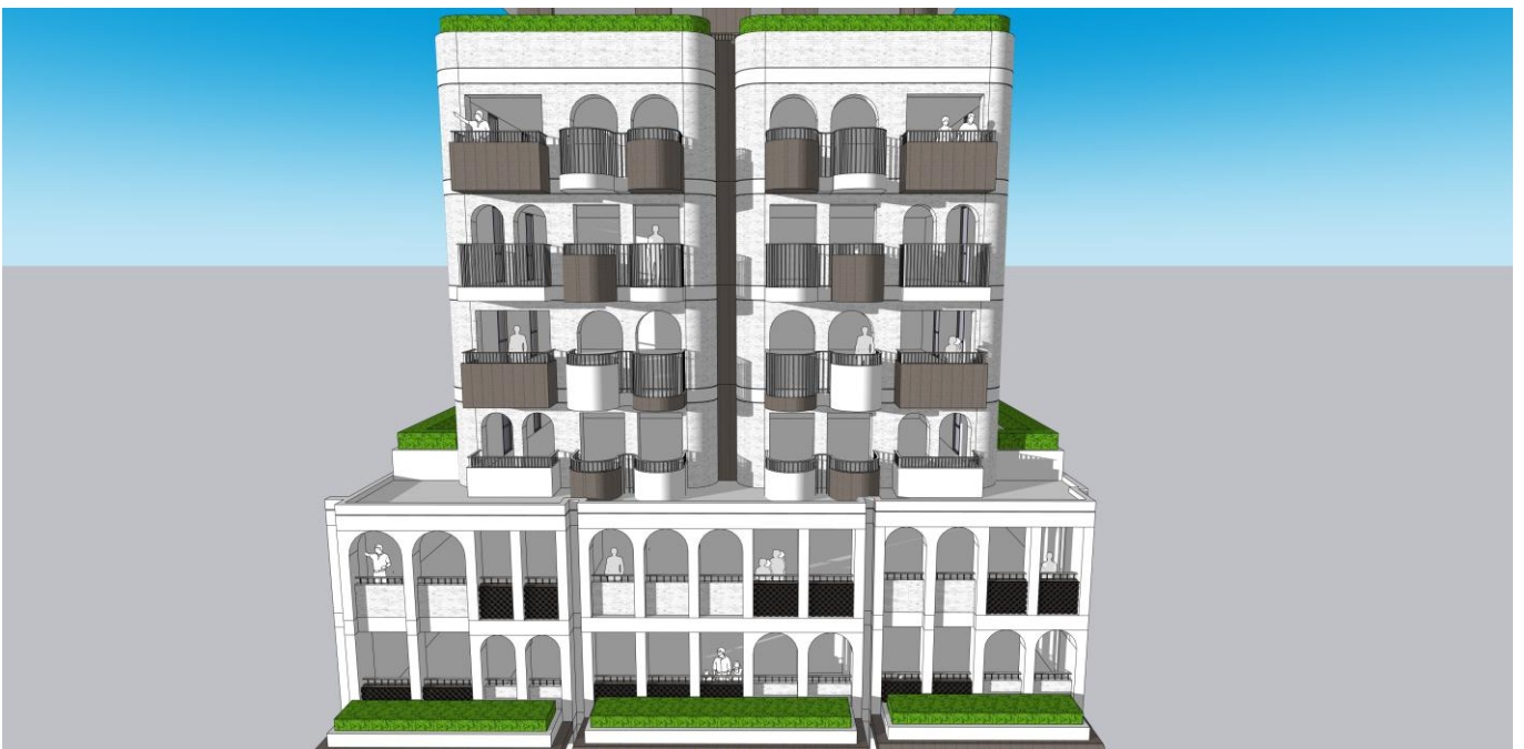
Above: upper level openings in a rhythm of arched and rectangular openings in similar proportions to podium wall openings.
