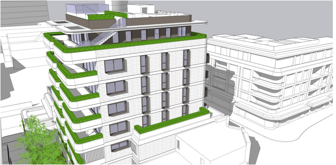
Above: east and west side facades with secondary windows with copper window shade frames
