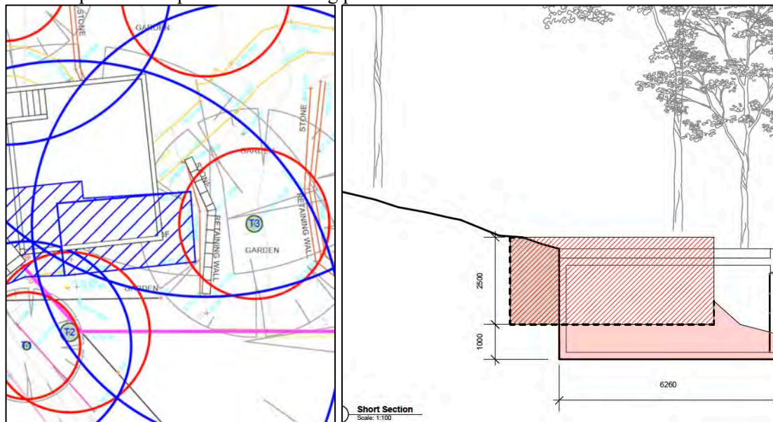
Figures 26 & 27: The layout depicting the existing garage and proposed double garage within the NRZ of Tree 3 (Left) and the cut and fill plan depicting the existing and proposed garage outlines. (Right). (Source: Site Plans by askerroberston design and construction dated 18/06/2025)
