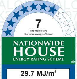
Predicted annual energy load for heating and cooling based on standard occupancy assumptions.
