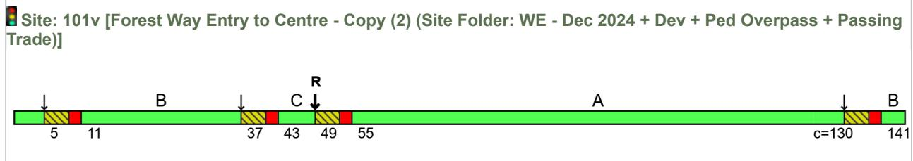
**Cycle Time = 130 seconds (Network User-Given Cycle Time)**
