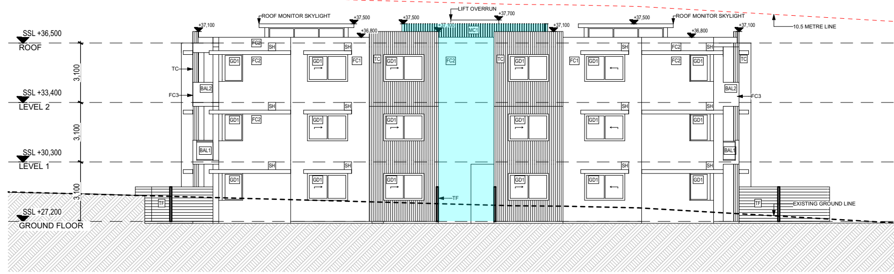
2 South Elevation - Building C Scale @ A1 = 1:200
