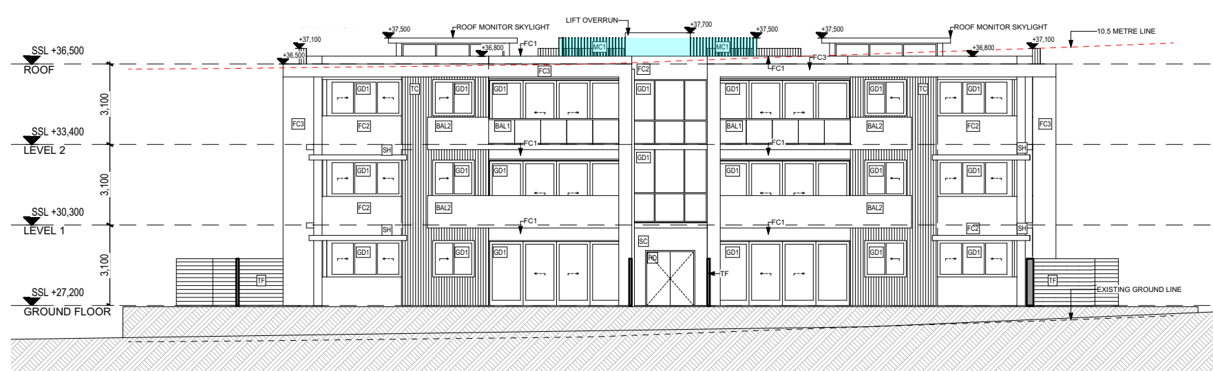
1 North Elevation - Building C Scale @ A1 = 1:200
