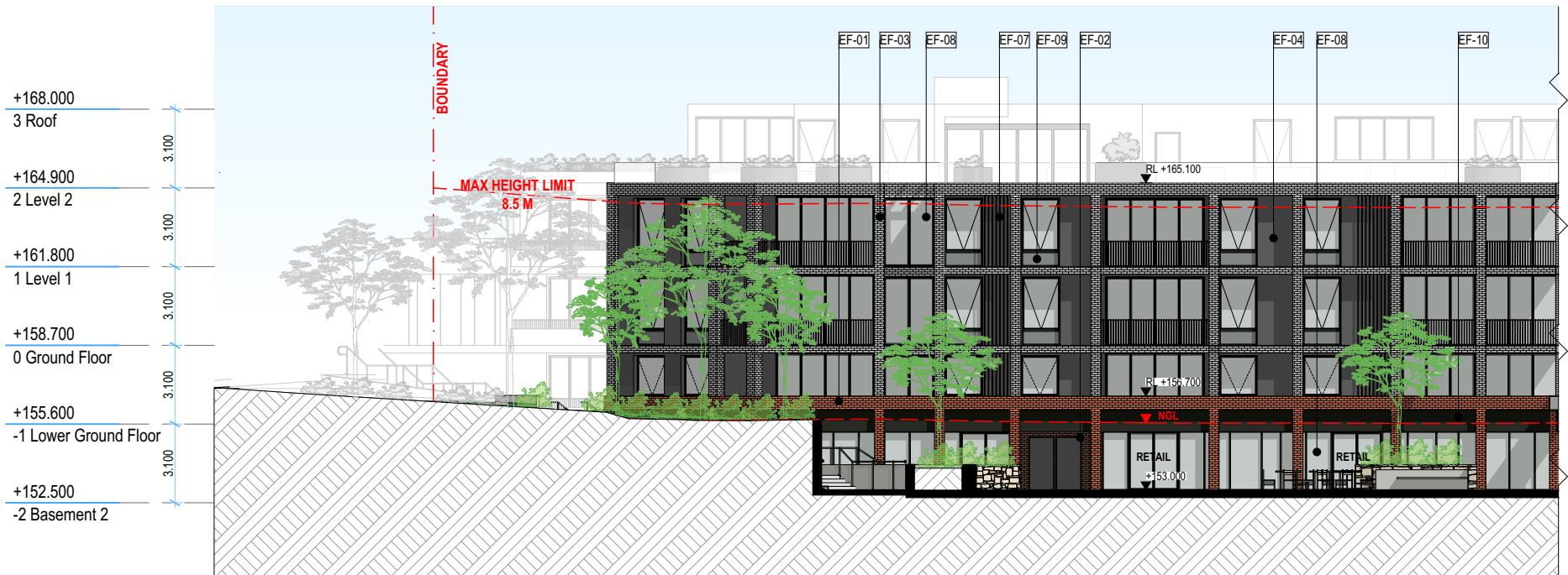
E-05 North Internal Elevation 1:250
