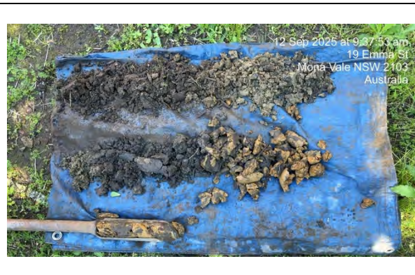
Photo 4: Subsurface soil profile of BH1.
