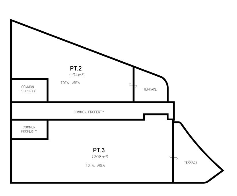
TERRACES ARE LIMITED IN HEIGHT TO 2.5 ABOVE THE UPPER SURFACE OF THE CONCRETE FLOOR THEREOF EXCEPT WHERE COVERED WITHIN THIS HEIGHT LIMIT.
