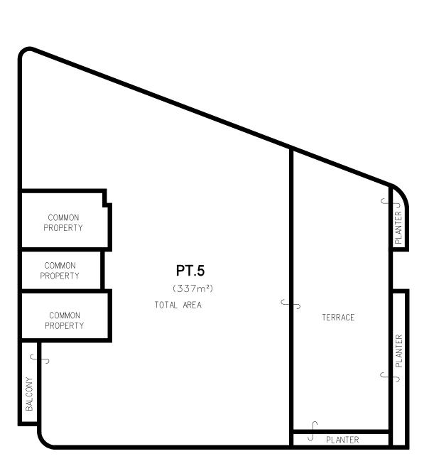
TERRACE, BALCONY & PLANTERS ARE LIMITED IN HEIGHT TO 2.5 ABOVE THE UPPER SURFACE OF THE CONCRETE FLOOR THEREOF EXCEPT WHERE COVERED WITHIN THIS HEIGHT LIMIT.
