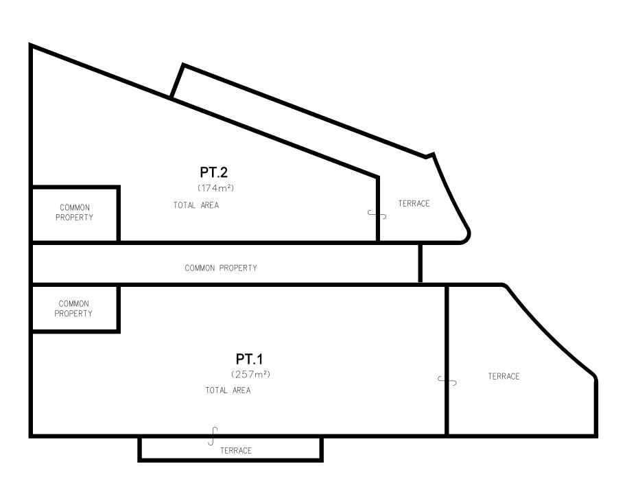
TERRACES ARE LIMITED IN HEIGHT TO 2.5 ABOVE THE UPPER SURFACE OF THE CONCRETE FLOOR THEREOF EXCEPT WHERE COVERED WITHIN THIS HEIGHT LIMIT.
