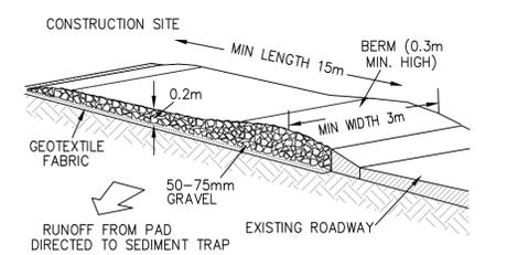
**NOTE:** WHEEL WASH OR SPRAY MAY BE REQUIRED DURING WET WEATHER. GRAVEL SHALL BE CLEANED/REMOVED WHEN THE EXPOSED HEIGHT OF THE GRAVEL IS LESS THAN 30mm.
