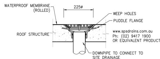
**PREFORMED OUTLET TO PARAPET OR BALCONY OVERFLOW**
