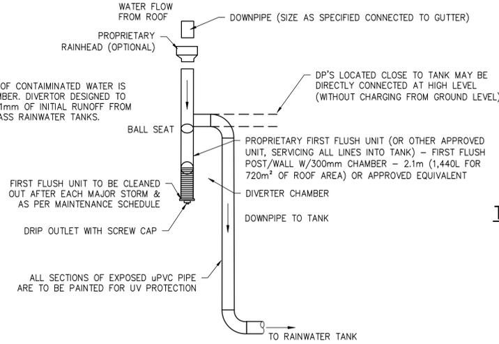
**TYPICAL WALL MOUNTED FIRST FLUSH DETAIL**
