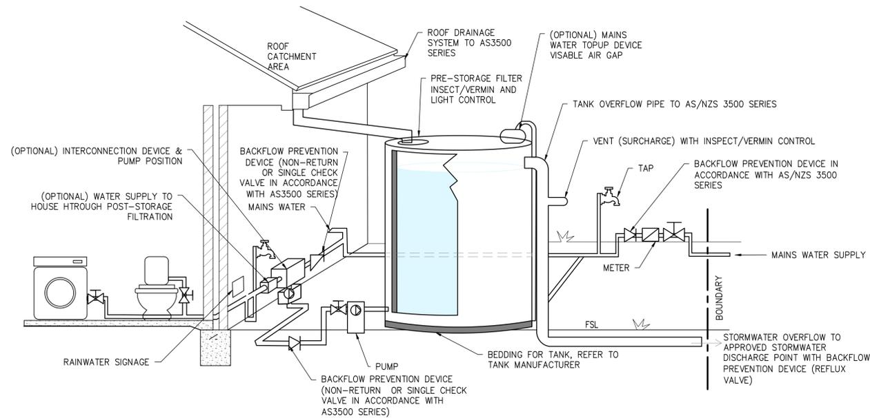
TYPICAL ABOVE-GROUND RAINWATER TANK INSTALLATION WITH MAINS WATER TOP-UP AND RAINWATER SUPPLIED TO APPLIANCES IN THE HOUSEHOLD (HB 230-2008)
