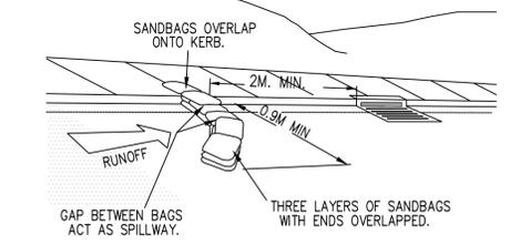
**GRAVEL KERB INLET SEDIMENT TRAP**
