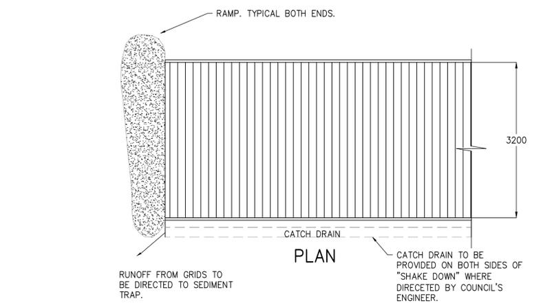
**NOTE:** WHEEL WASH OR SPRAY MAY BE REQUIRED DURING WET WEATHER
