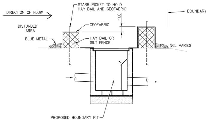
**SEDIMENT TRAP CONSTRUCTION SPECIFICATION:**
