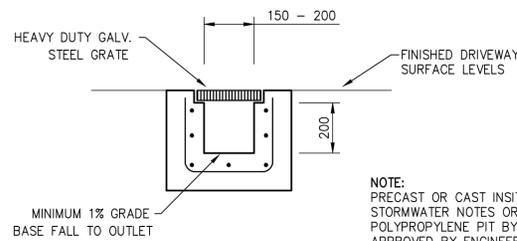
NOTE: PRECAST OR CAST INSITU PIT. REFER STORMWATER NOTES OR PROVIDE ALTERNATE POLYPROPYLENE PIT BY MANUFACTURER IF APPROVED BY ENGINEER
