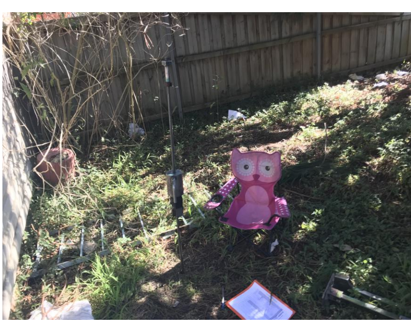
Photograph 6 DCP test at location of BH3/DCP3 within front garden
