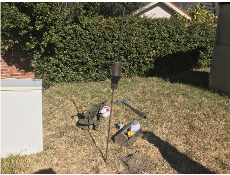
Photograph 4 Dynamic Cone Penetrometer (DCP) Test and drilling at location of DCP2 within rear garden
