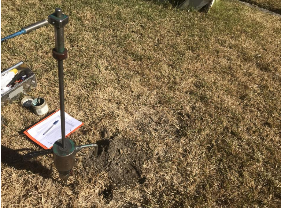
Photograph 5 DCP test in progress at location of BH1/DCP1 within rear garden
