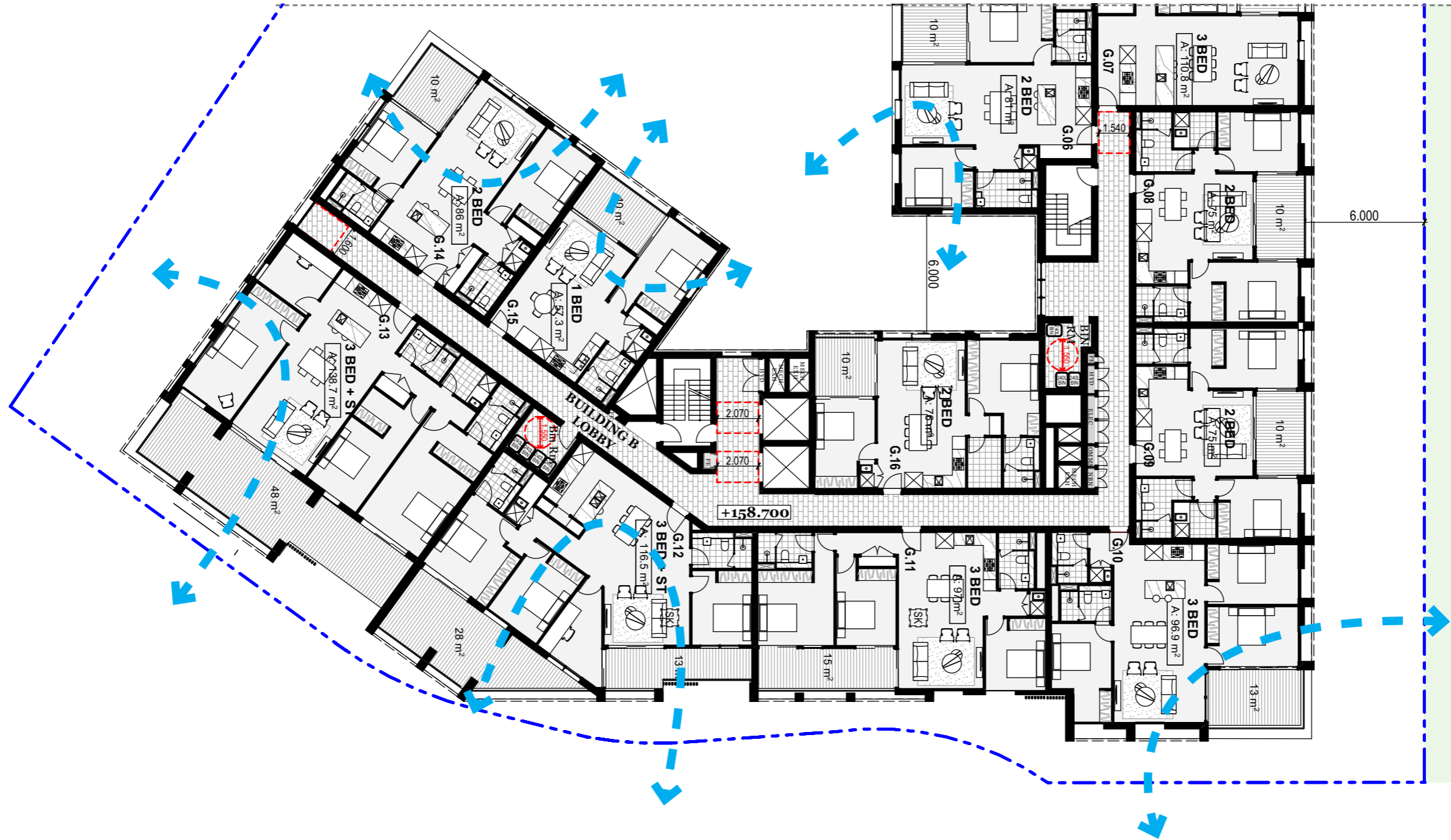
Ground Floor Cross Ventilation Study
