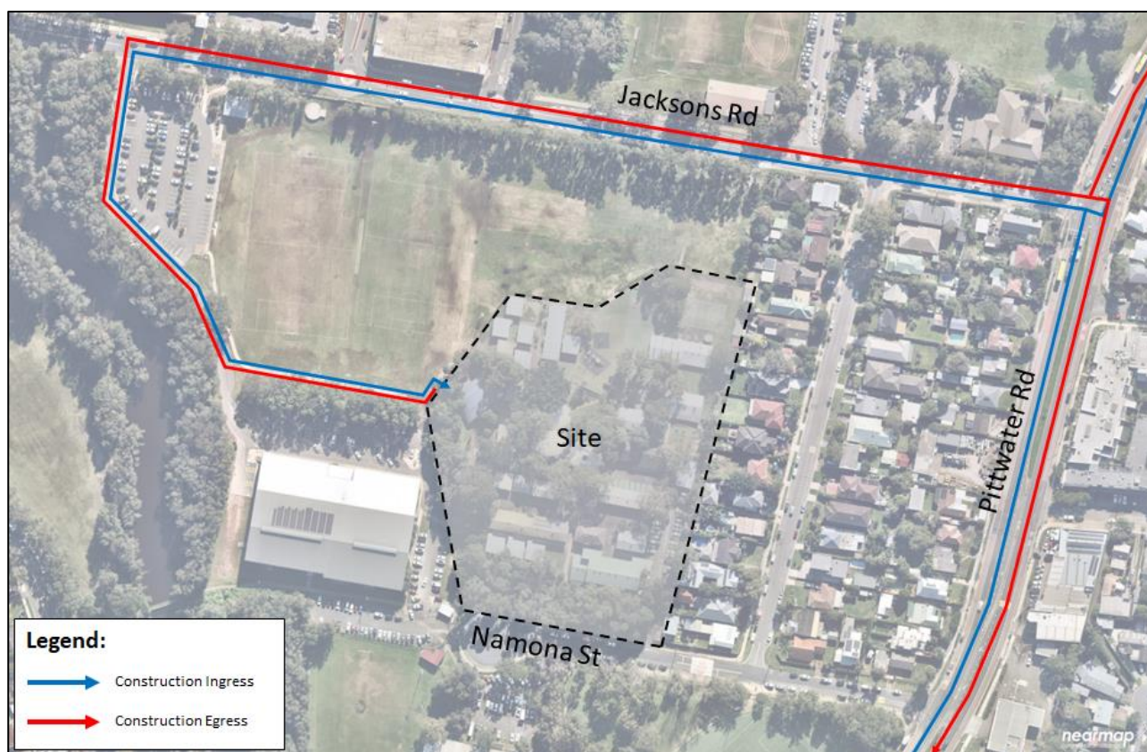
Figure 9: Construction Vehicle Haulage Routes
