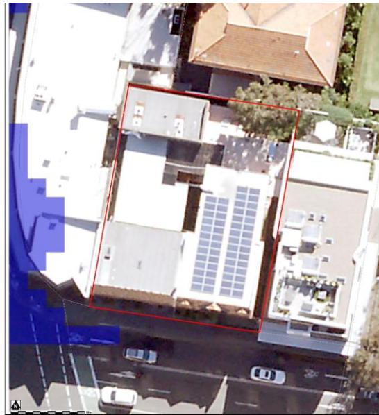
Figure 5.3 – 1% AEP Peak Flood Extent (Manly to Seaforth Flood Study, Cardno, doc number NA49913018, dated 22nd February 2019)
