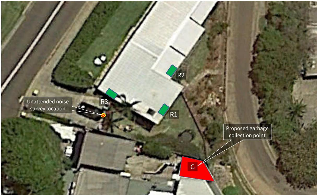
Figure 2. Proposed garbage collection point and noise-sensitive receiver locations (Image source – Google Earth)
