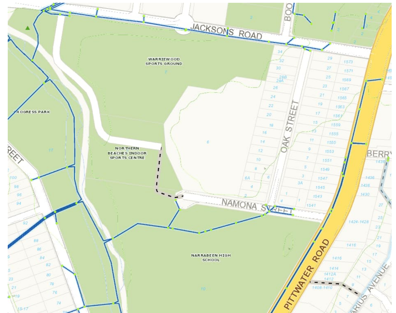
Figure 3: Stormwater system (Source: NBC Stormwater Map)
