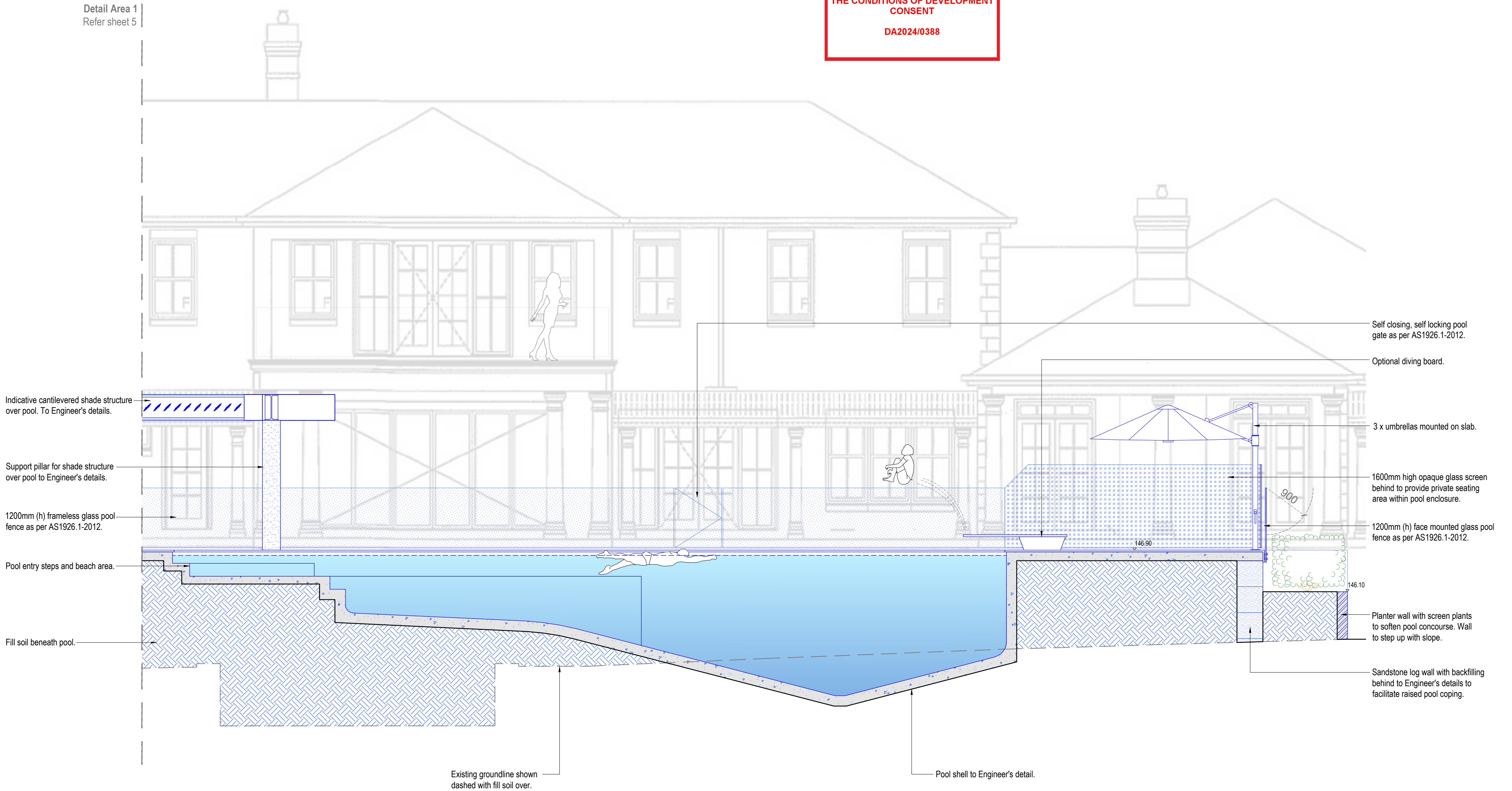
Sectional Elevation BB - Detail Area 2 - Pool Scale 1:50
