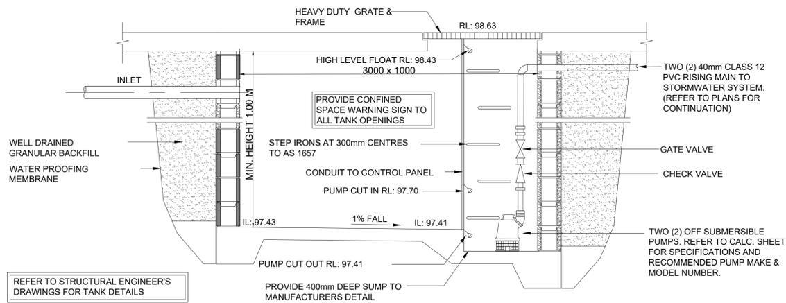
**PUMP-OUT TANK SECTION DETAIL**
