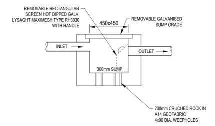
**TYPICAL SILT ARRISOTOR PIT DETAIL**
