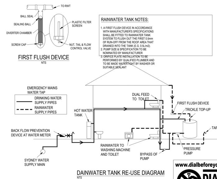
**RAINWATER TANK RE-USE DIAGRAM**
