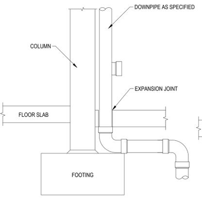
**SUFFICIENT CLEARANCE FROM TOP OF COLUMN FOOTING TO PAVEMENT SLAB**
