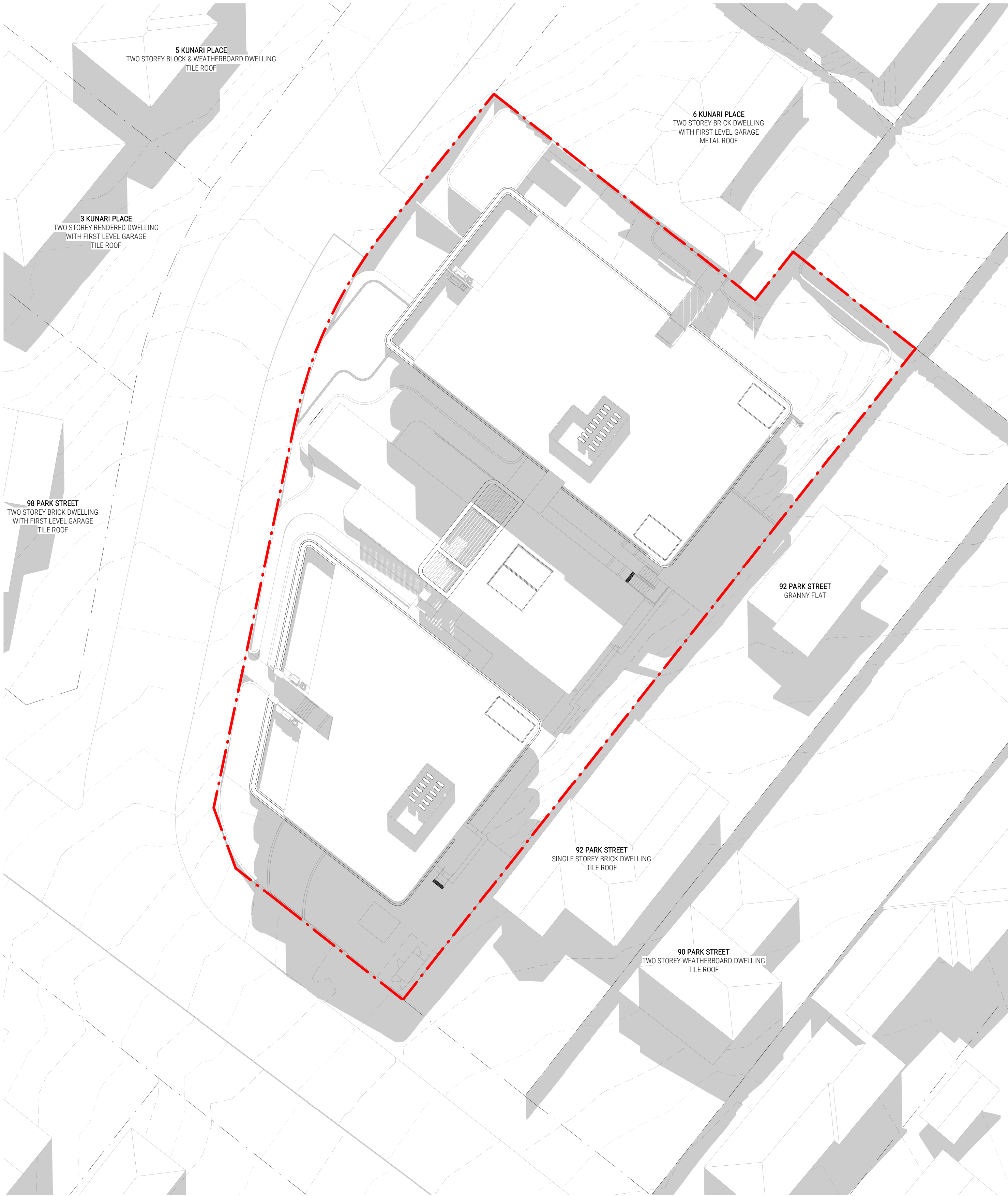
2 PROPOSED SHADOW DIAGRAM - 12PM JUNE 21ST DA502/ 1:250 @ A1
