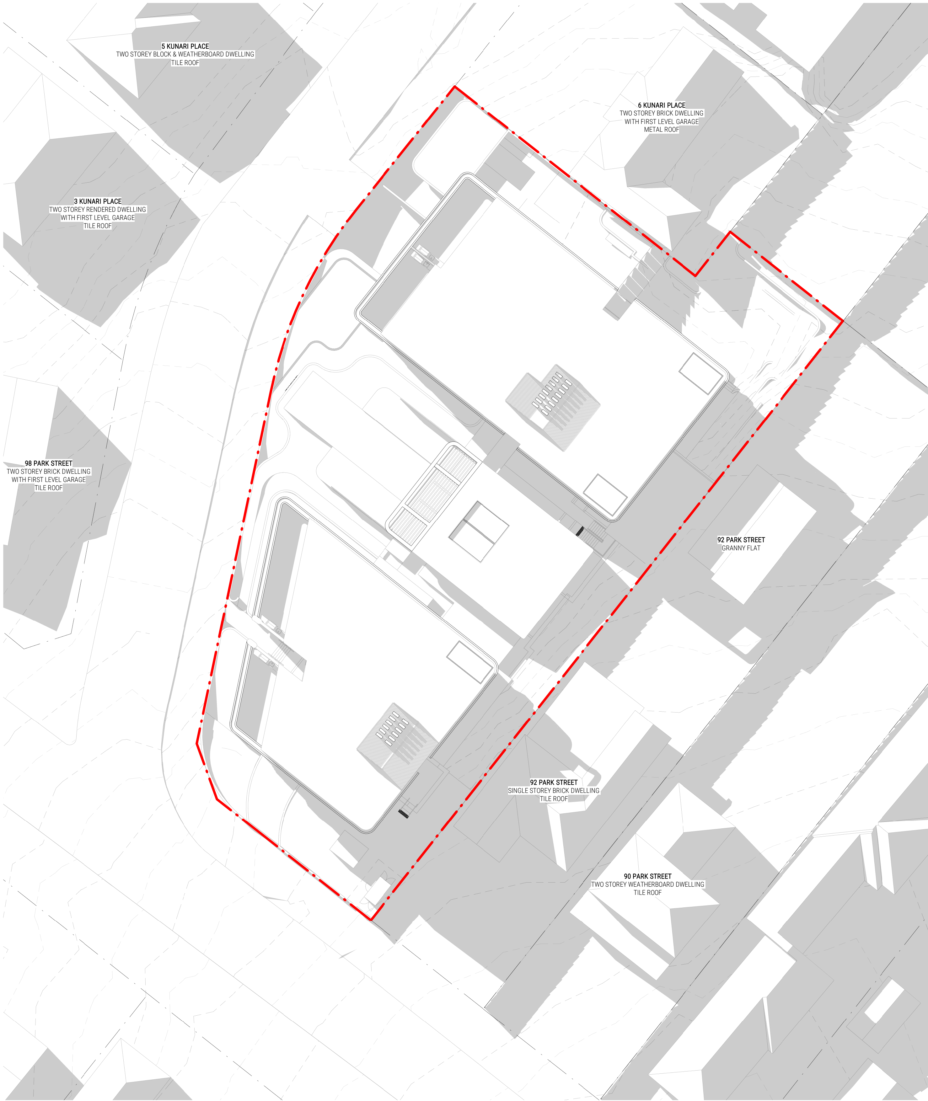
2 PROPOSED SHADOW DIAGRAM - 3PM JUNE 21ST DAS03/ 1:250 @ A1
