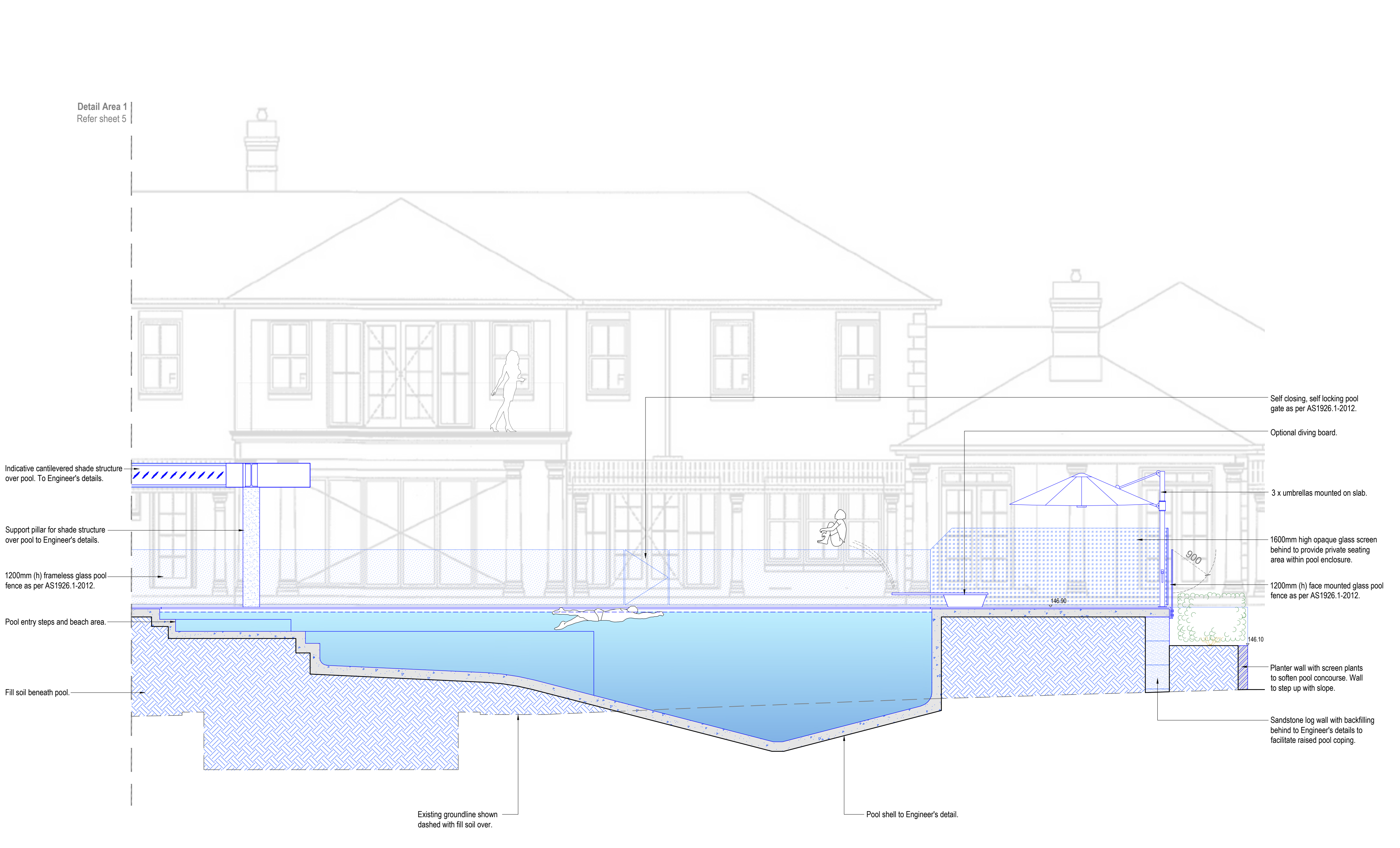
Sectional Elevation BB - Detail Area 2 - Pool Scale 1:50
