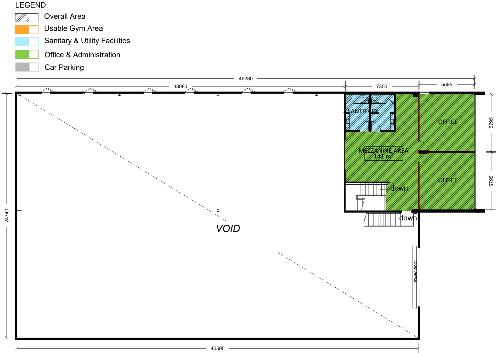
MEZZANINE FLOOR AREA STUDY SCALE: 1:200
