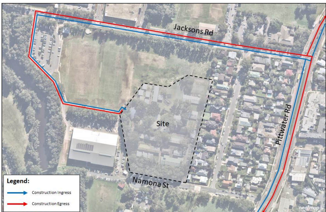
Figure 9: Construction Vehicle Haulage Routes
