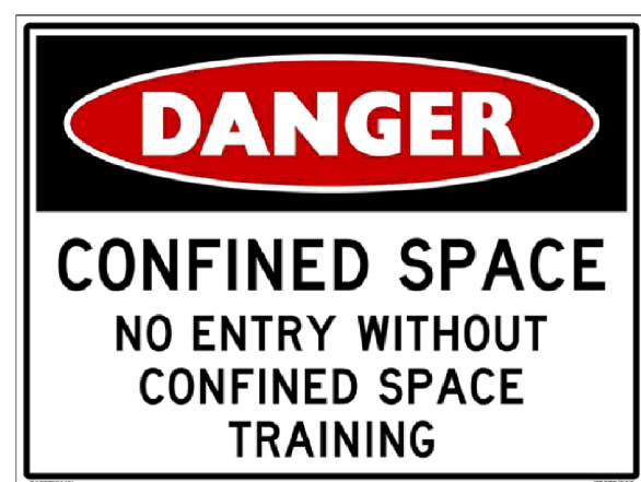
7 DETAIL - CONFINED SPACE SIGN TO BE PLACED INSIDE OSD TANK & BASEMENT PUMPOUT PIT NTS
