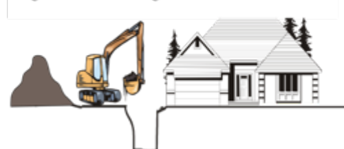
Fig. 11 De-stabilizing house foundations
