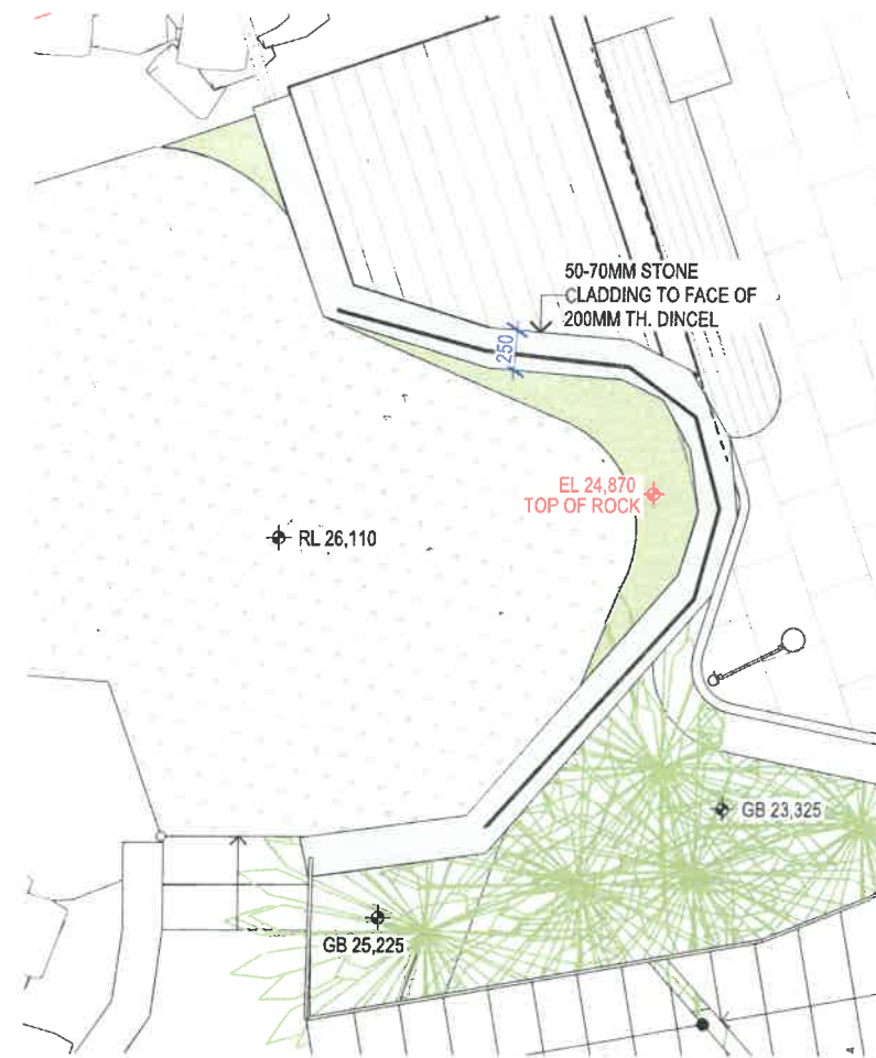
A RETAINING WALL PLAN 1:50
