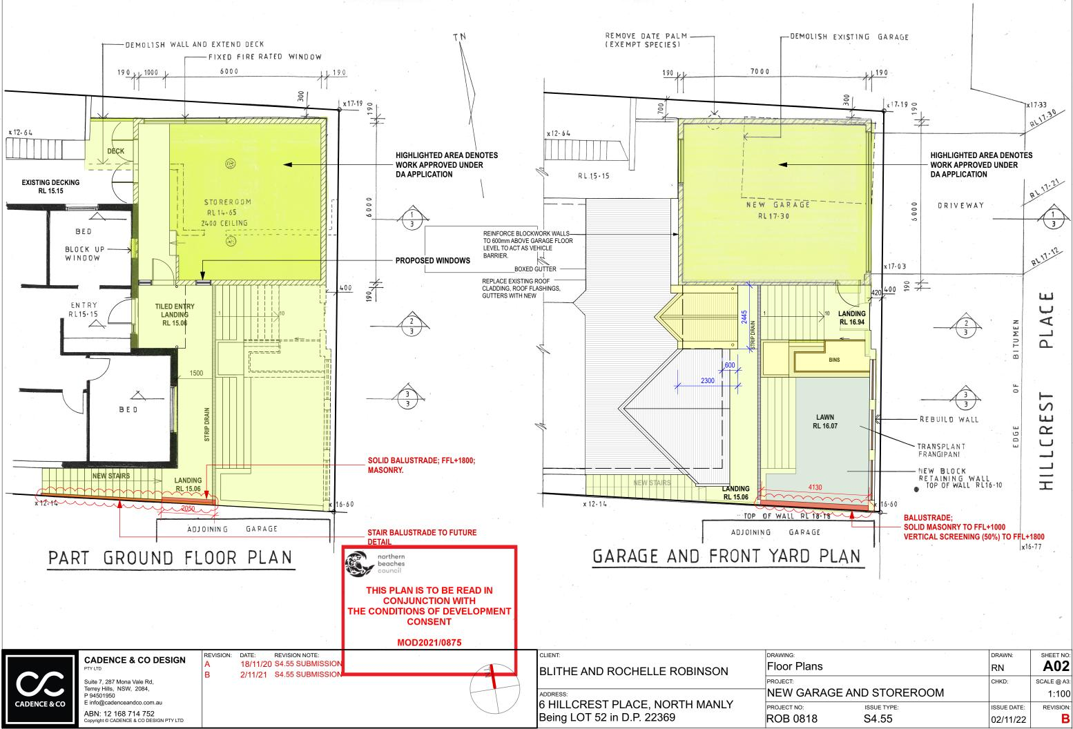
GENERAL NOTES: ALL RL'S SHOWN ARE FINISHED LEVELS, BUILDER TO PROVIDE SET DOWNS & ALLOWANCES AS REQUIRED. ALL OPENING DIMENSIONS ARE NOMINAL, BUILDER TO CHECK SIZES ON-SITE BEFORE ORDERING WINDOW AND DOOR UNITS.
