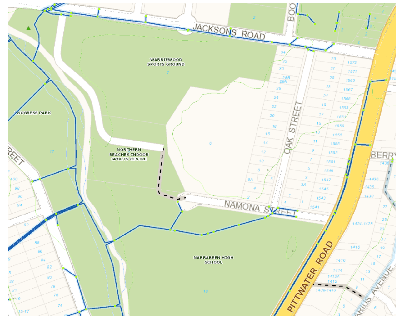
Figure 3: Stormwater system (Source: NBC Stormwater Map)
