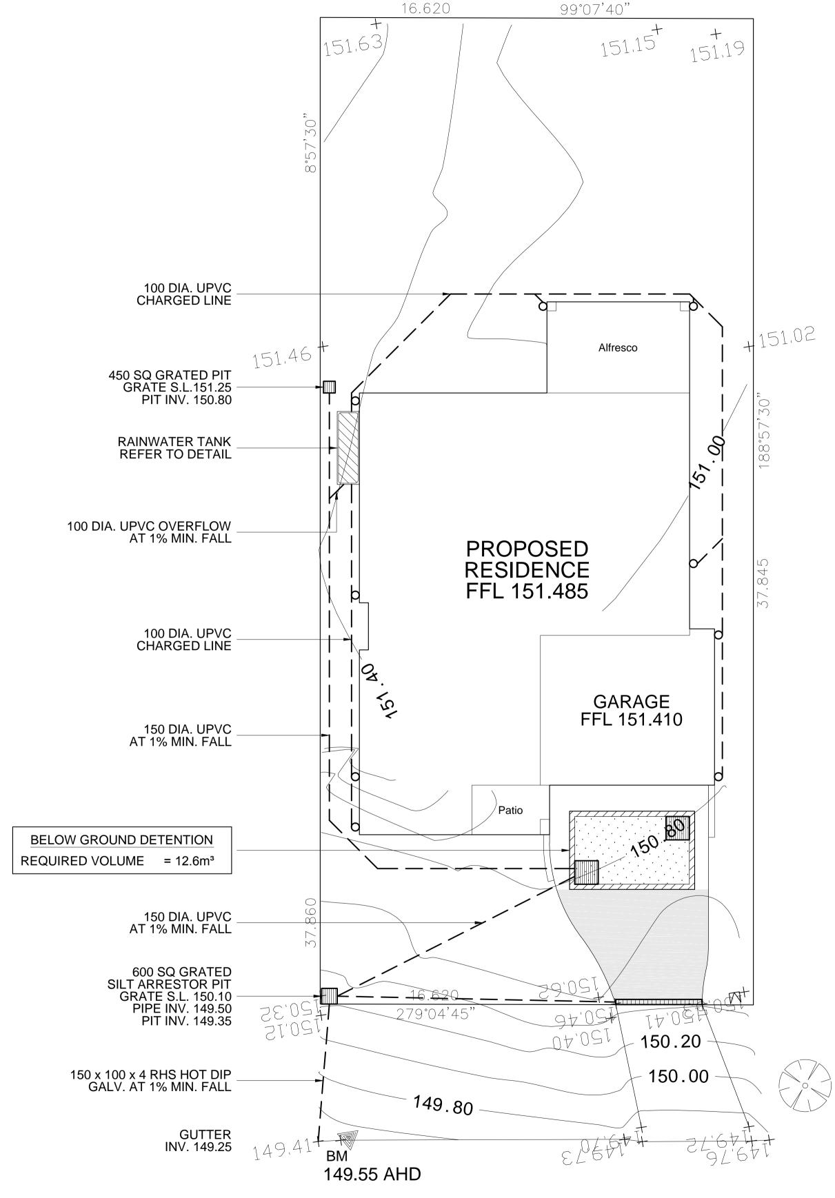
SHADING INDICATES IMPERVIOUS AREA BYPASSING OSD
