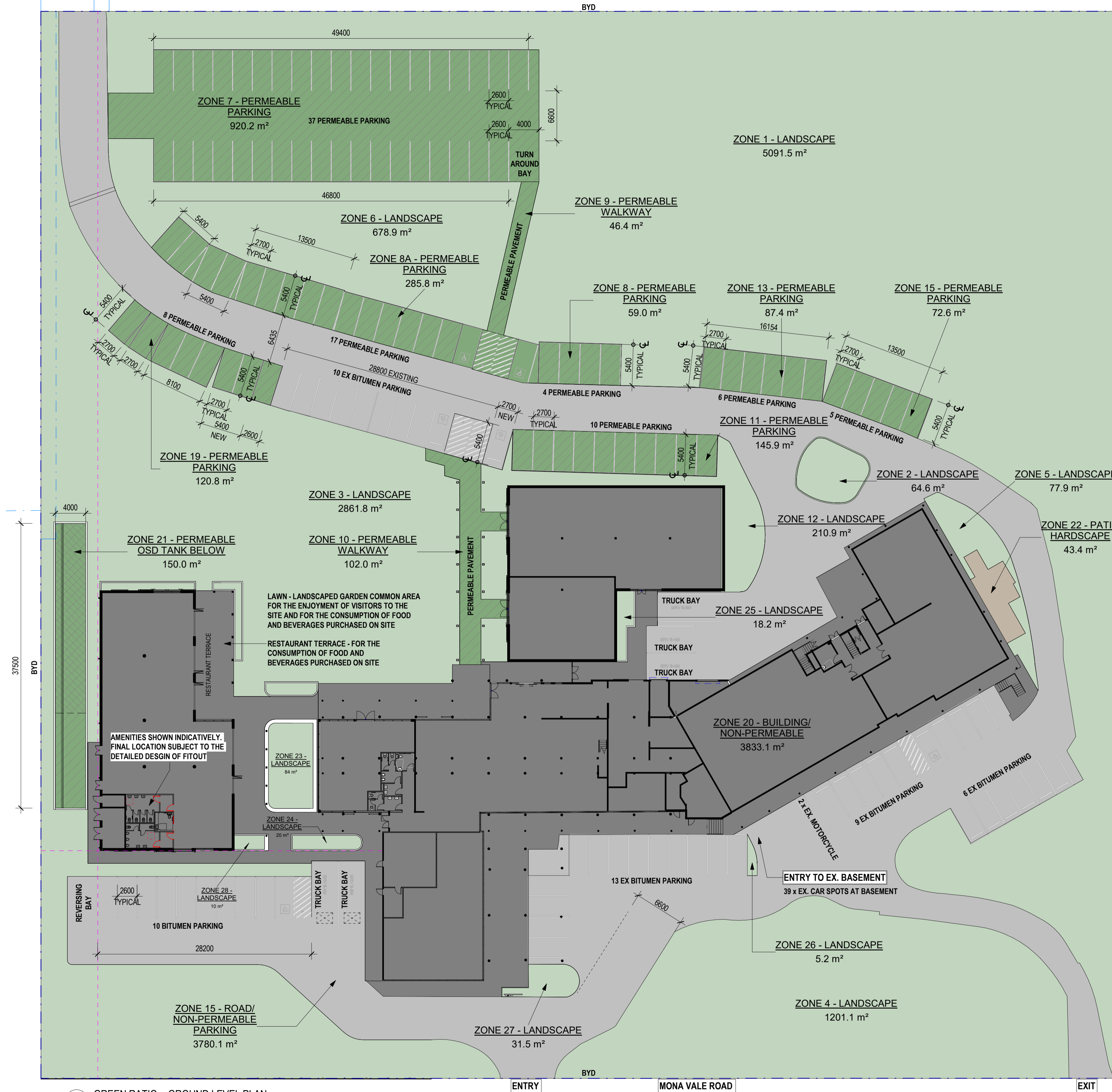
1 GREEN RATIO - GROUND LEVEL PLAN 1:300
