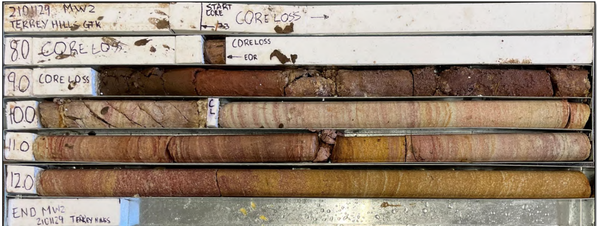
Borehole MW2 – NMLC coring completed from 7.30 to 13.00 mbg.
