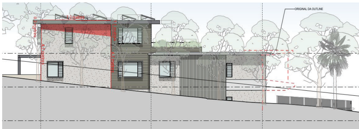
North Elevation envelope breach (source Gartner Trovato)
