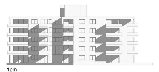
SHADOW COMPARISON BETWEEN APPROVED DA AND NEW PROPOSAL USING DESIGN CUBICLE MODEL OF NEIGHBOURING PROPERTY
