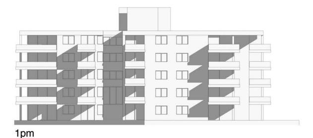
SHADOW CAST BY NEW PROPOSAL + SELF-SHADOWING USING DESIGN CUBICLE MODEL OF NEIGHBOURING PROPERTY
