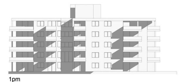
SHADOW CAST BY APPROVED DA + SELF-SHADOWING USING DESIGN CUBICLE MODEL OF NEIGHBOURING PROPERTY
