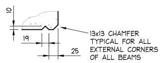
NOTE: ALL DRIP GROOVES, CHAMFERS AND REGLETS AS PER ARCHITECTS DETAILS. MAINTAIN CORRECT COVER AT THESE LOCATIONS. SECTIONS NOTED AS SIMILAR MAY HAVE SLAB THICKNESSES THAT VARY.
