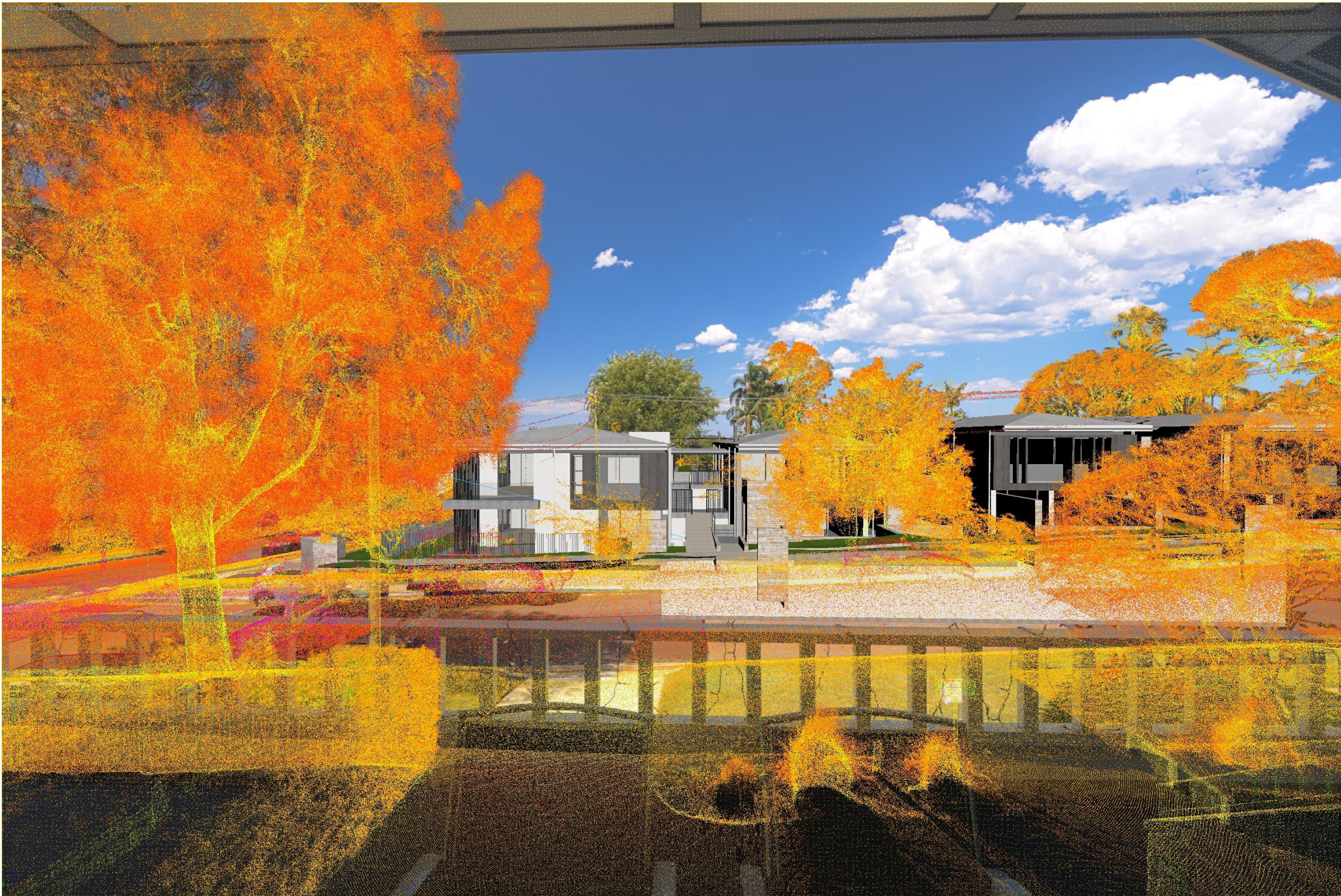
1V5A2017hdr - No.38 : Proof showing surveyed point cloud overlaid on photograph with proposal
