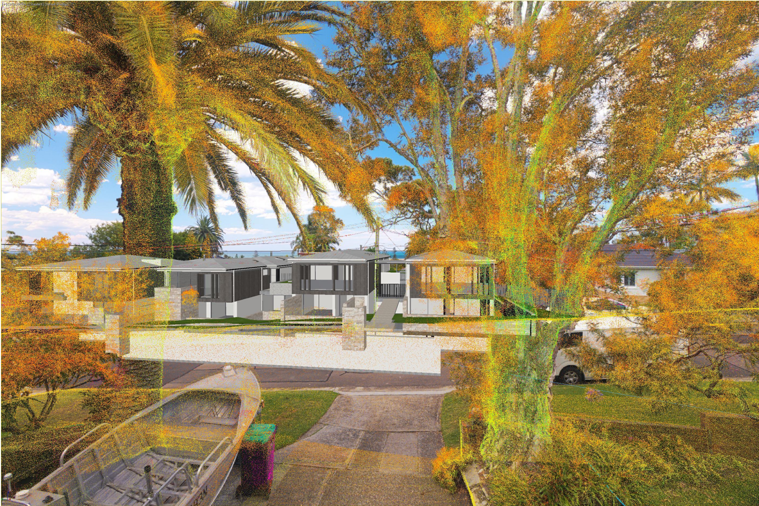
1V5A2065hdr - No.34 : Proof showing surveyed point cloud overlaid on photograph with proposal
