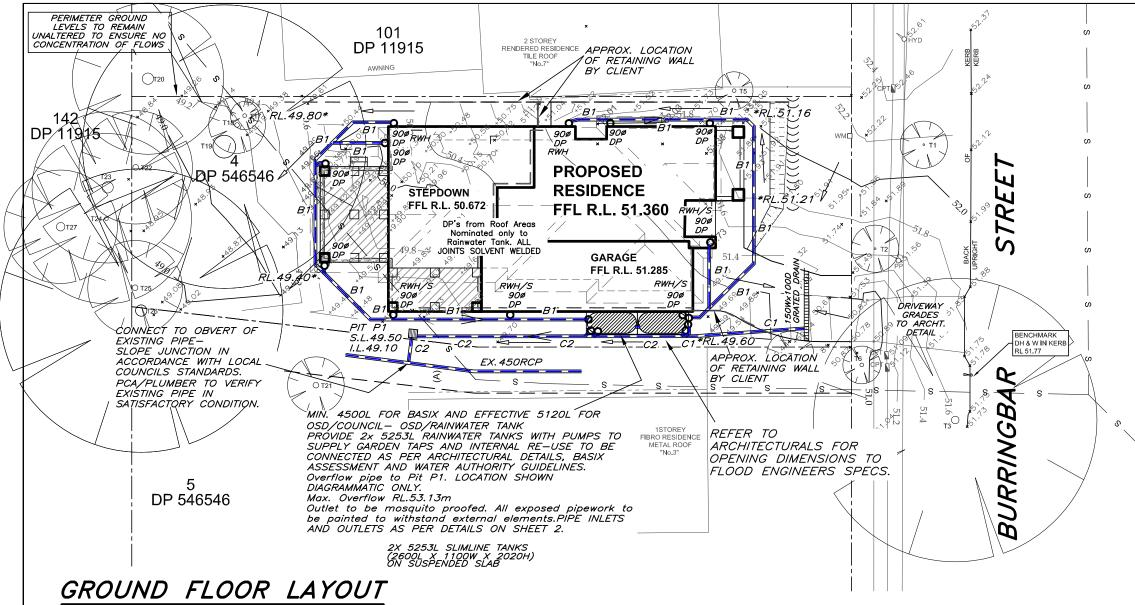
REFER TO SHEET 2 FOR RAINWATER TANK DETAILS. LEAF GUTTER GUARDS OR SIMILAR SCREENING RECOMMENDED TO ALL GUTTERS. WHSA HAZARD IDENTIFICATION:
