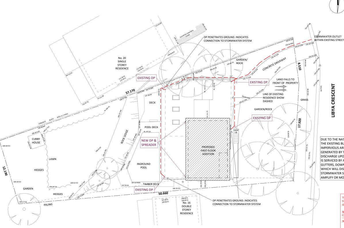
PROPOSED STORMWATER PLAN 1:200
