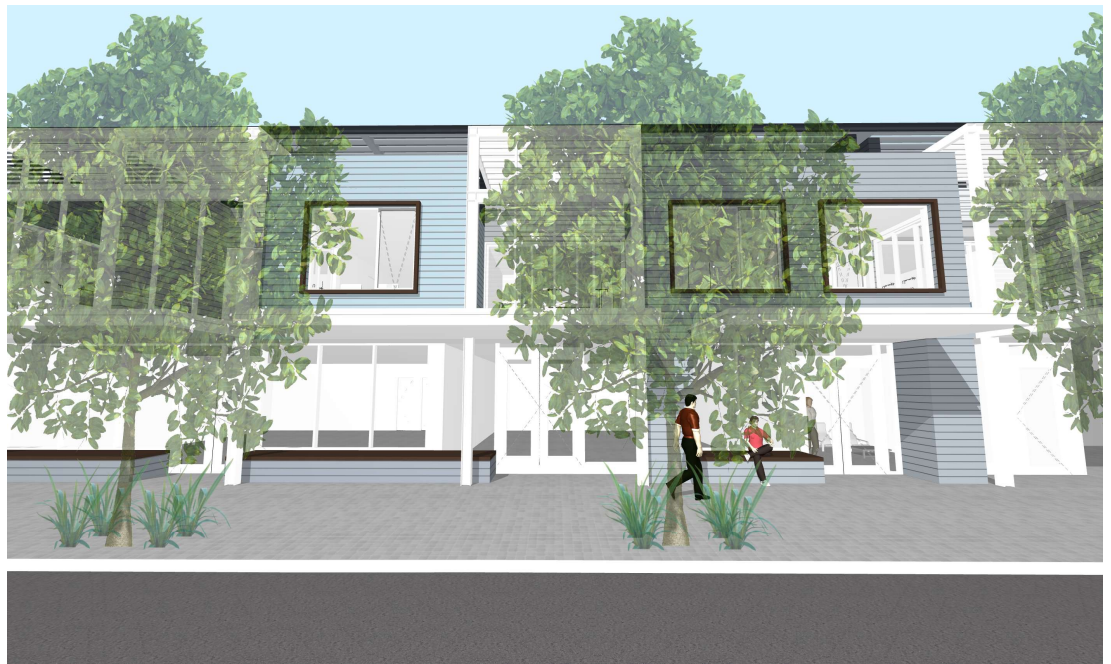
Figure 13: View of west façade facing Pittwater Road, showing weatherboard cladding, steel framed wintergardens, awnings, and street planting.
