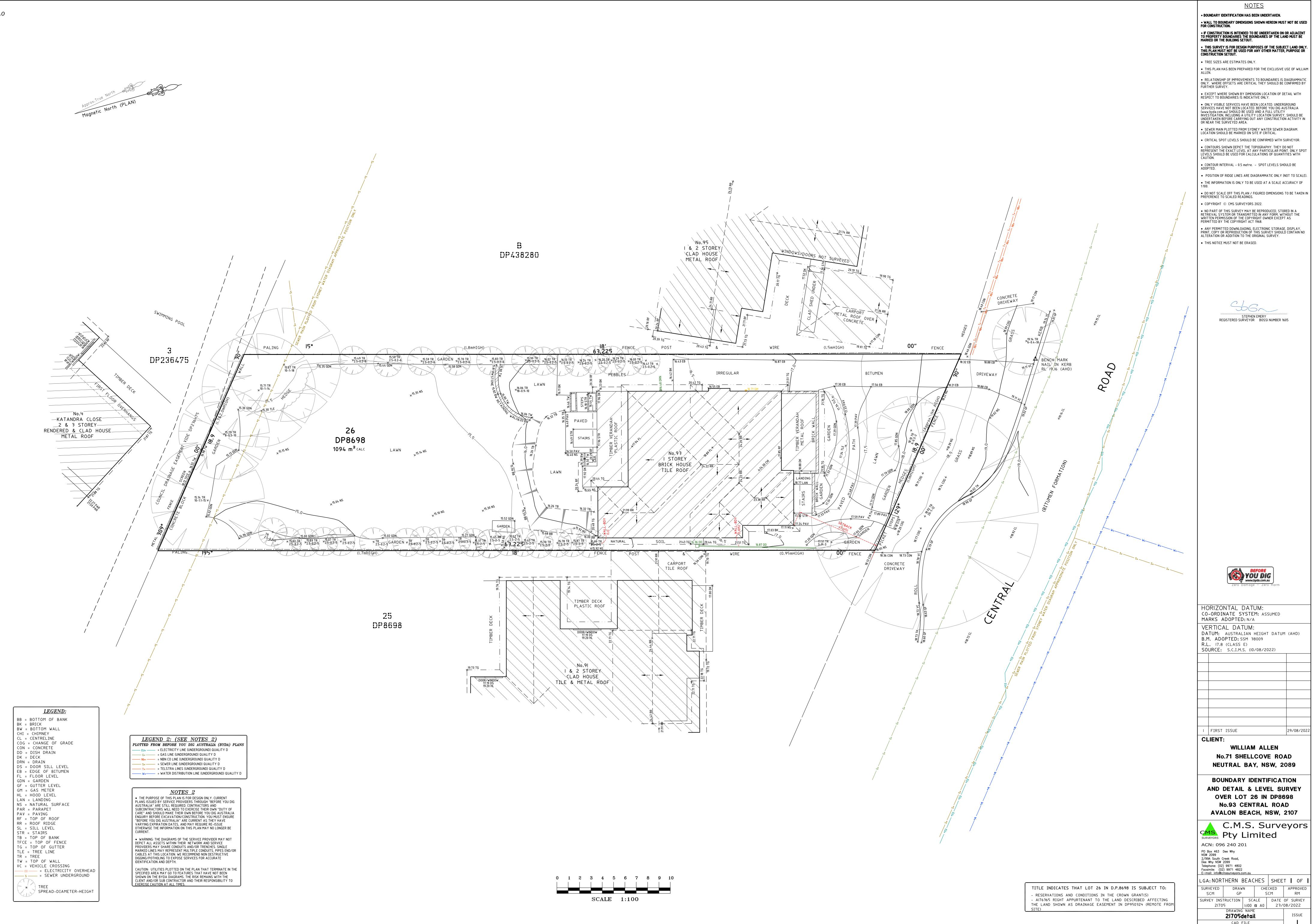
WALL TO BOUNDARY DIMENSIONS SHOWN HEREON MUST NOT BE USED FOR CONSTRUCTION. IF CONSTRUCTION IS INTENDED TO BE UNDERTAKEN ON OR ADJACENT TO PROPERTY BOUNDARIES THE BOUNDARIES OF THE LAND MUST BE MARKED OR THE BUILDING SETOUT.
