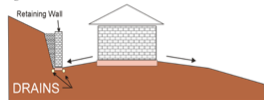
Fig. 5 Well Drained Sites
