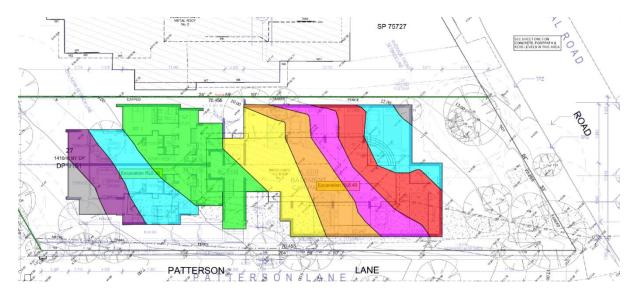
Compared to previous design, there is now no longer any need for the excavation to be staged. Additionally, there has now been a reduction in the amount of estimated volume of excavated material.
