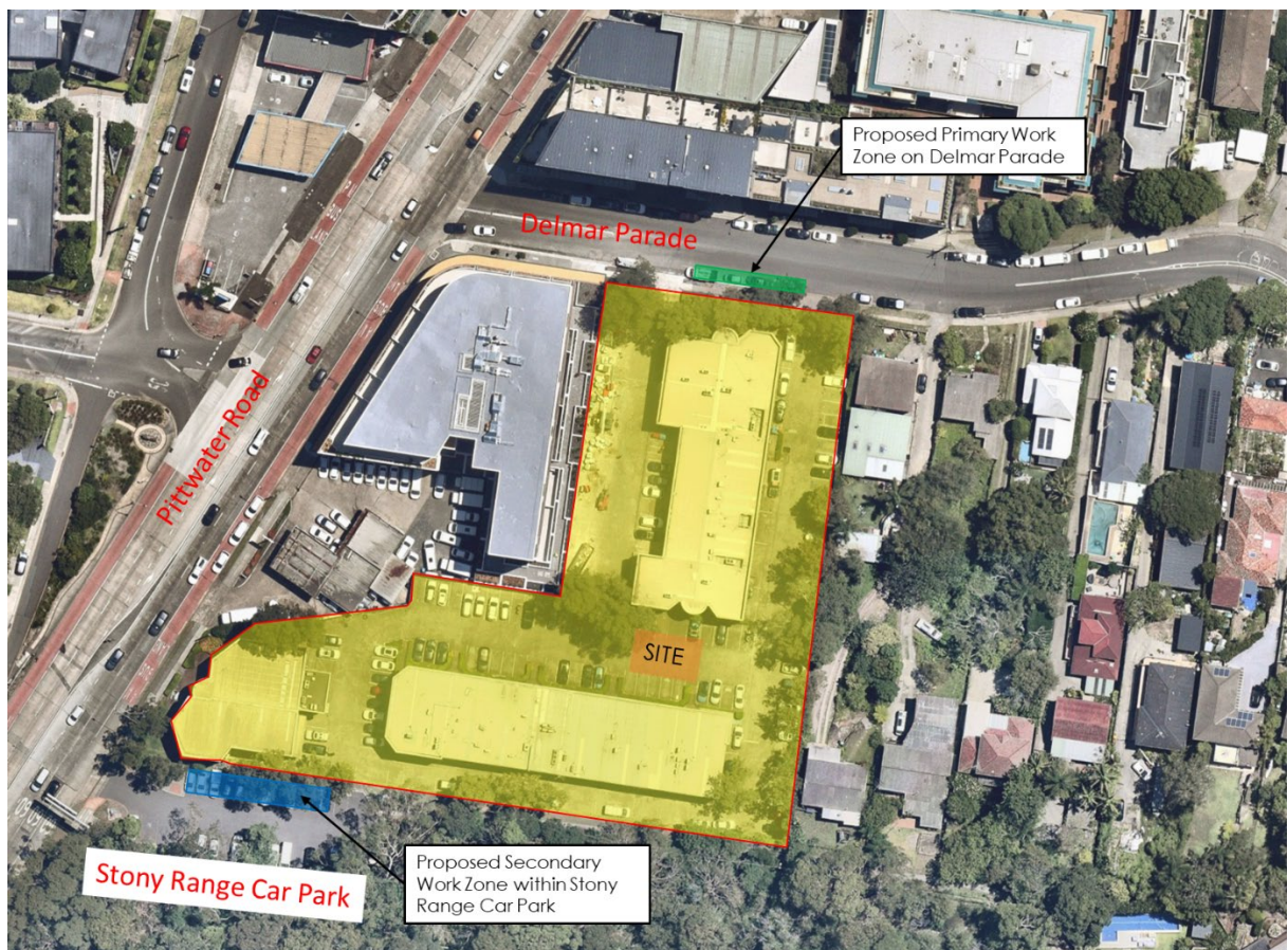
Figure 3.4: Delmar Parade Works Zone Location
