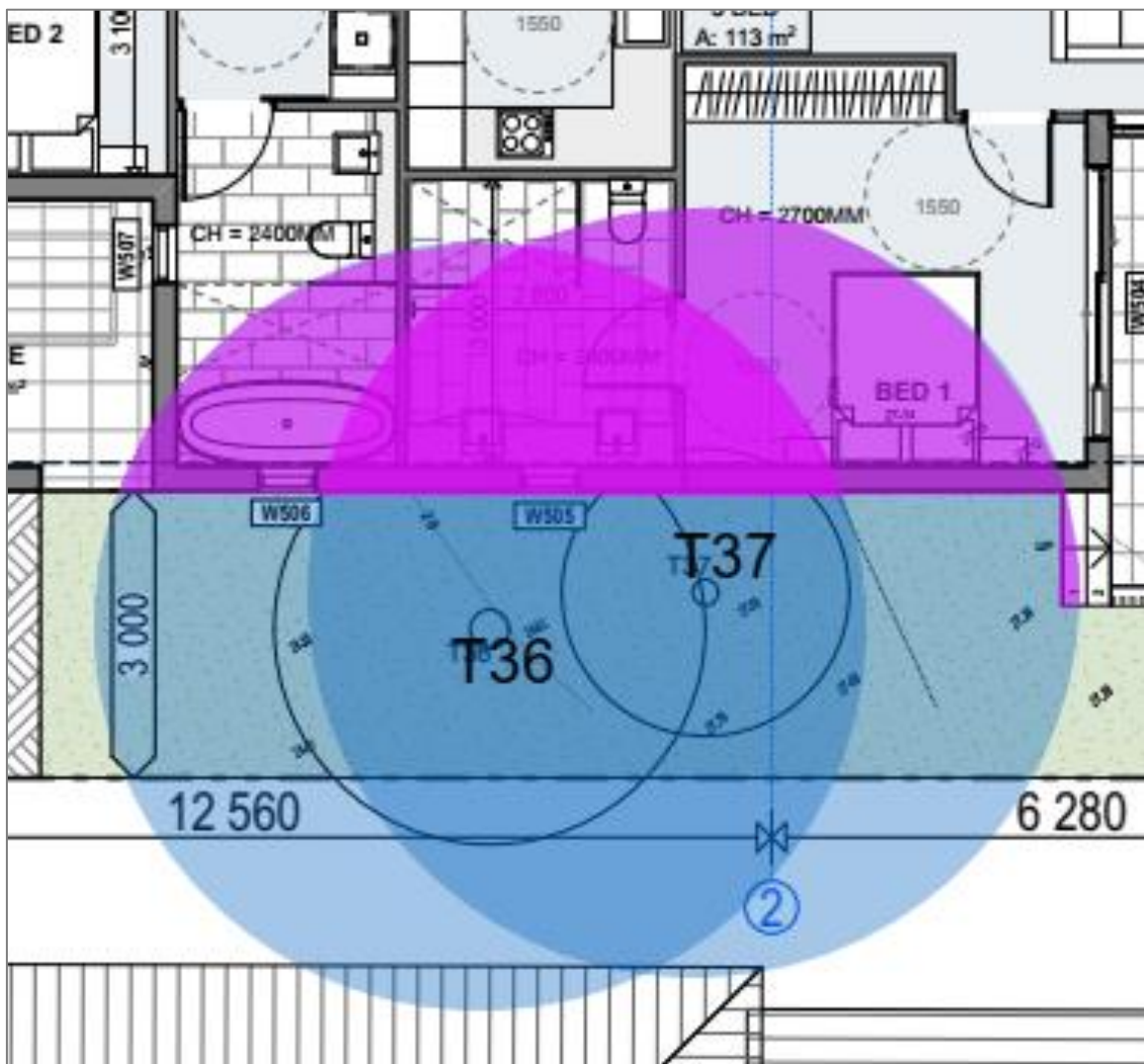
Figure 9 –Tree 36 & 37 encroachment calculation – Excerpt of Level 01 Plan, Project 2306, dwg no. A.06, 23/10/23 authored by Gartner Trovato Architects. Red hashed circle indicates SRZ, blue shaded circle denotes the TPZ. Pink shading indicates encroachment. NOT TO SCALE. Marked up by C Hughes.
