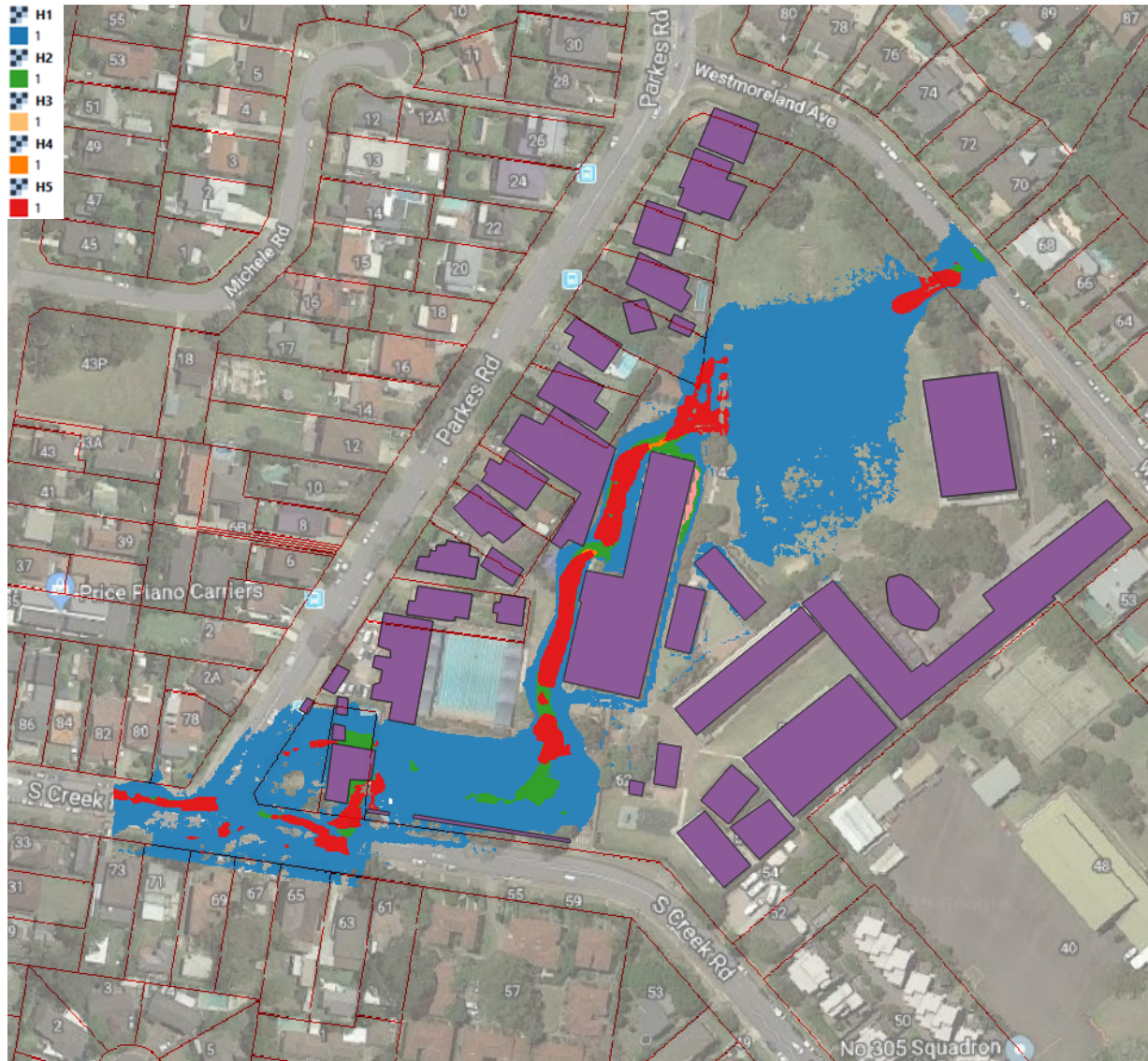
Figure 19 - Pre-development, 1% AEP (blocked), Flood Hazard
