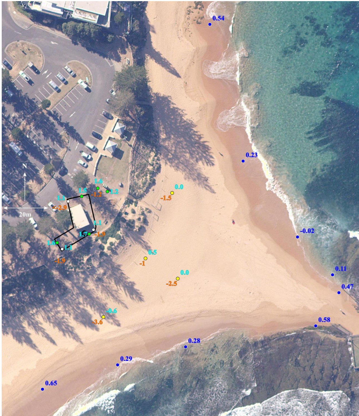
Figure 12: AHD levels of top of clay (light blue) and top of bedrock (orange) in boreholes, and probed bedrock AHD levels (dark blue) in JK Geotechnics geotechnical investigations, with proposed building roof outline in black (17 August 2018 aerial photograph)
