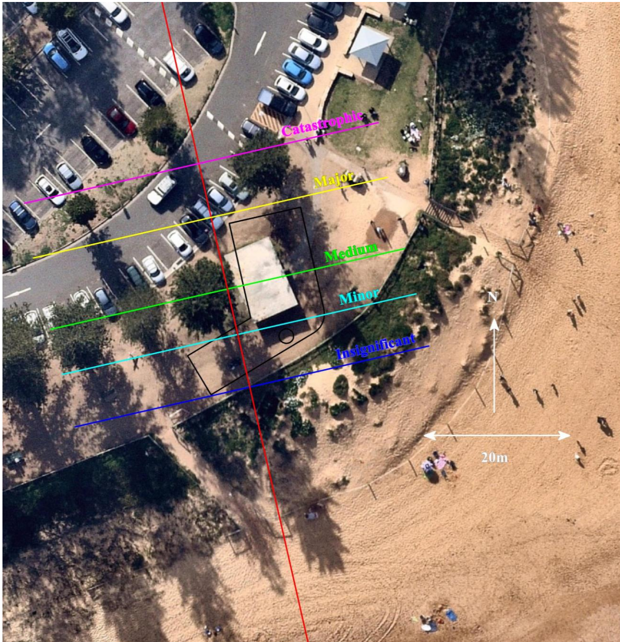
Figure 15: Designated consequence locations to match five AGS (2007a, b) consequence descriptors (aerial photograph taken 2 August 2020)
