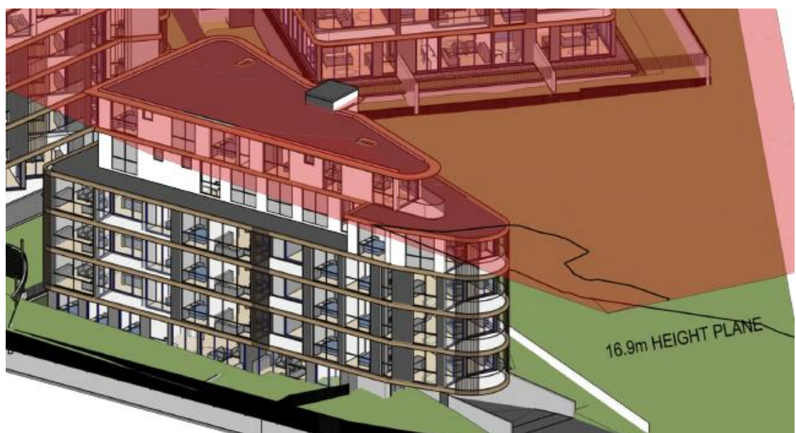
Figure 13 – Plan extract of 16.9 metre building height blanket diagram depicting minor non-compliant projecting elements on Building C.
