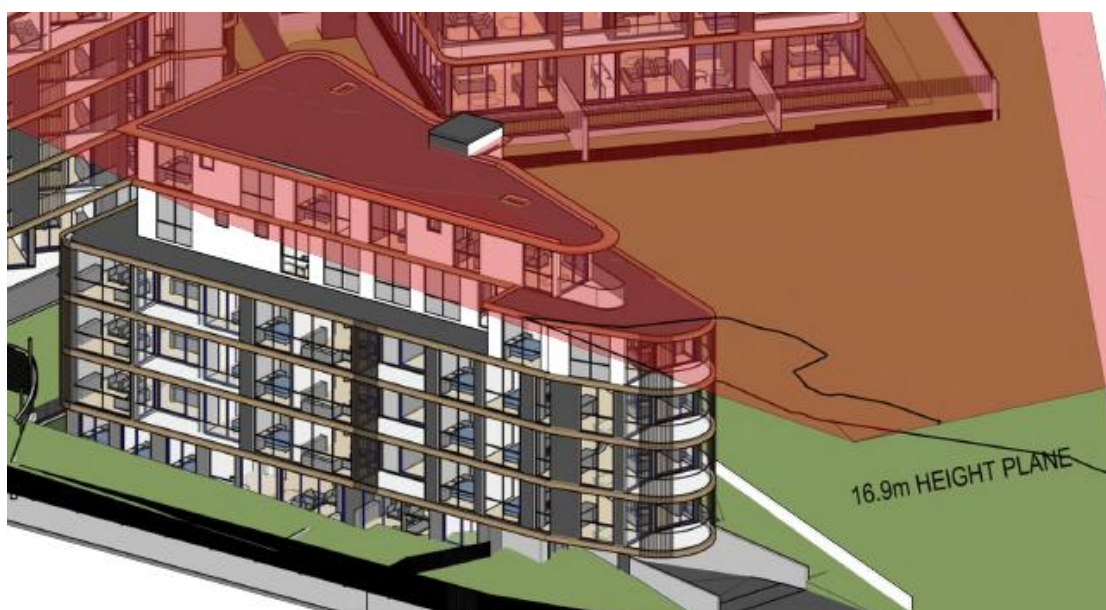
Figure 16 – Plan extract of 16.9 metre building height blanket diagram depicting minor non-compliant projecting elements on Building C.
