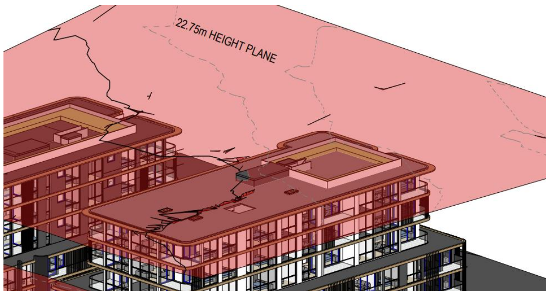
Figure 15 – Plan extract of 22.75 metre building height blanket diagram depicting minor non-compliant projecting element on Building A.
