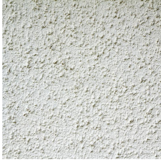
RM01 RENDERED MASONRY PAINTED, SMOOTH FINISH
