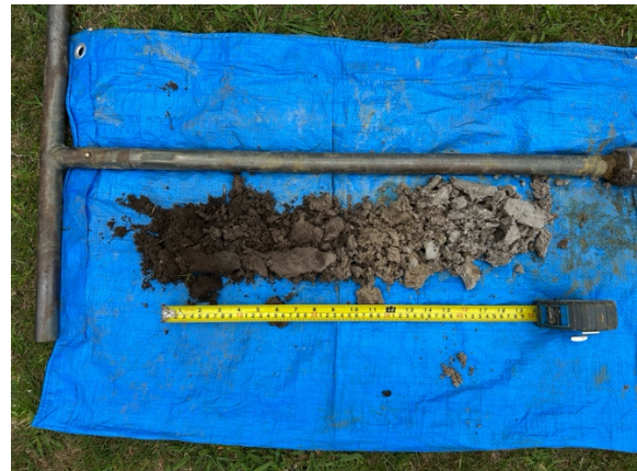
Photo 4: Subsurface soil profile seen in BH2.
