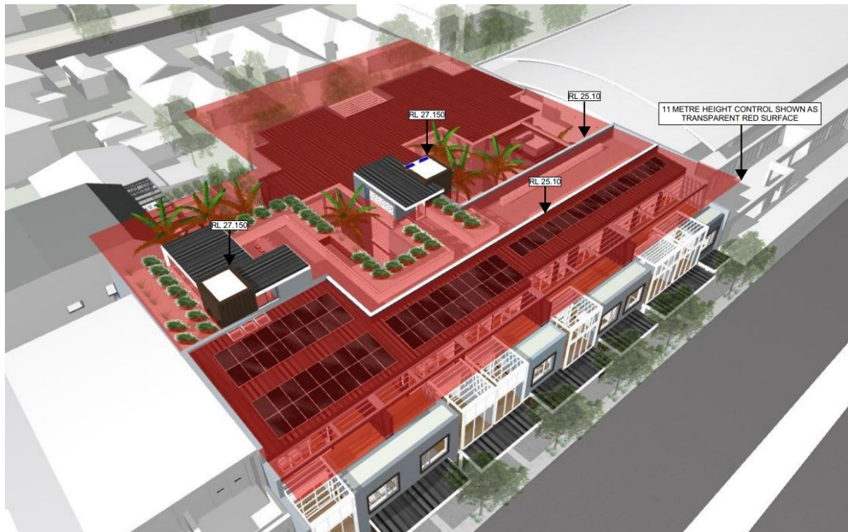
Figure 1 – Building height blanket diagram showing non-compliant building height elements
