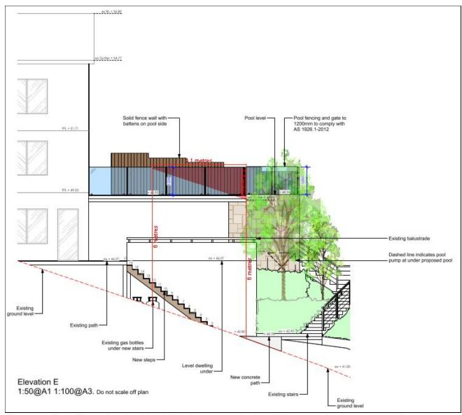
Figure 1. East Elevation (red highlighting numerical building envelope non-compliance)
