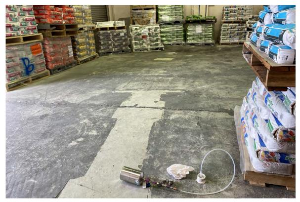
**Photograph 14:** Soil vapour sampling location SV2.
